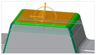
PTC Creo FMX helps you quickly edit geometry to your desired position by pushing and pulling the 3D Dragger.
