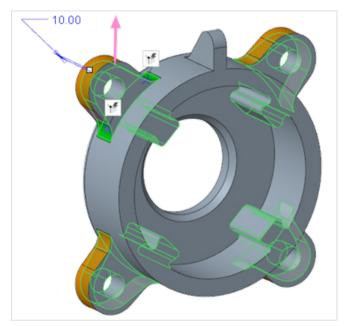
Recognize patterns of geometry in imported parts and propagate geometric changes to the pattern members with PTC Creo FMX.
